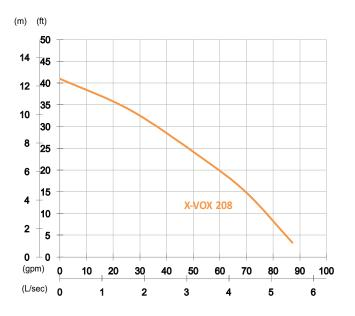
Shaft Speed: 2850 rpm Outlet: 50mm, 2in
